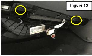
**8.** Undo the 5 x glove box screws and grasp and remove the glove box. Refer figure 14 & 15.
