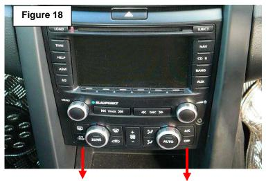
11. After facia is removed undo the 4 screws at the following positions and remove the AHU. Refer figure 19.
