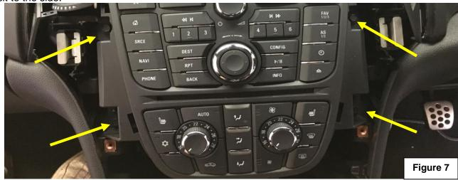
**5.** Once stereo is visible remove 2 x bolts and remove stereo from cavity.
