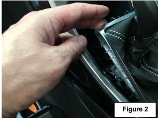
2. With gear shift surround lifted locate the 2 screws either side of the center panel and remove both screws. After removing lift and remove surround entire surround. Gear shift surround can be guided
