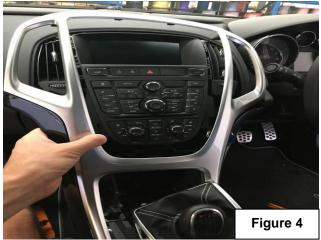
3. With stereo surround removed unclip both sides of vent assy to expose the bolts. Refer figure 5 & 6.
