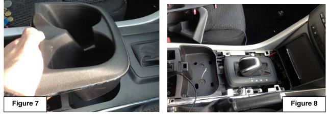
6. Remove the centre storage compartment by grasping and pulling towards the rear of the vehicle. Refer figure 9.
