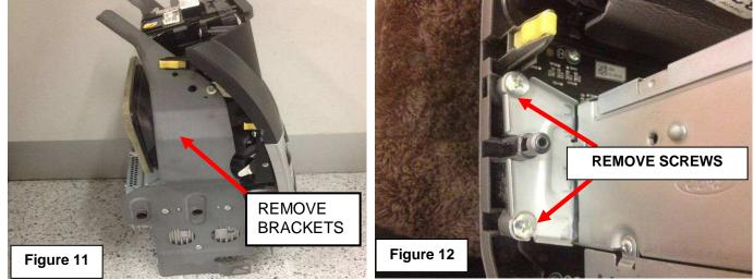
11. Remove the 2 x screws from either side of the audio module holding it in place and remove the cable tie attached to the top of the chassis holding the cable in place.
