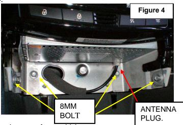
3. Grasp ICC and pull towards the rear of the vehicle and remove from vehicle.
